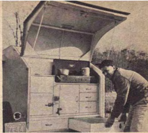
Compact arrangement of kitchen area shows stove, ice box, water tap, storage drawers.
