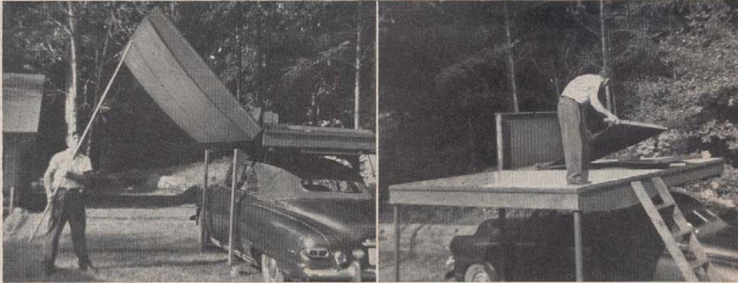
Is gently lowered to rest on two slip-in legs. Walls are next. From stack in the box . . .
