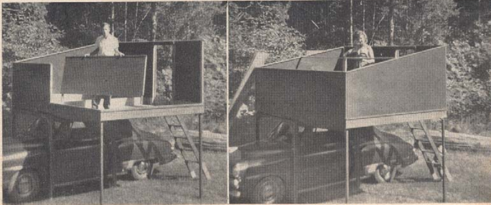
They slip into grooves and sockets on rim. Bolted-together walls hold roof support . . .
