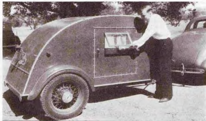
Louis Rogers of Pasadena, designer and builder, demonstrates the novel window bracket. Normally, it is worked from the inside.
