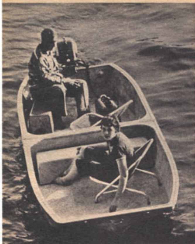
BOAT-CAMPER-TRAILER. Thirteen-foot fiber glass boat folds up to 77-inch trailer, is put in water by removing wheels, unfolding hull sections. Aluminum rods hold sections apart to sleep two in 200-pound rig. Aqua Trailers, Inc., Spokane, Wash. Price: $695.
