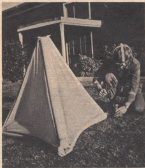
INFLATABLE MARKER for helicopter landing sites is being tested by U.S. Marines. It can also be used as emergency marker for mountaineers, rangers or sailors at sea.
