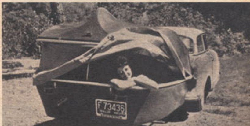
BOAT-CAMPER-TRAILER. Thirteen-foot fiber glass boat folds up to 77-inch trailer, is put in water by removing wheels, unfolding hull sections. Aluminum rods hold sections apart to sleep two in 200-pound rig. Aqua Trailers, Inc., Spokane, Wash. Price: $695.
